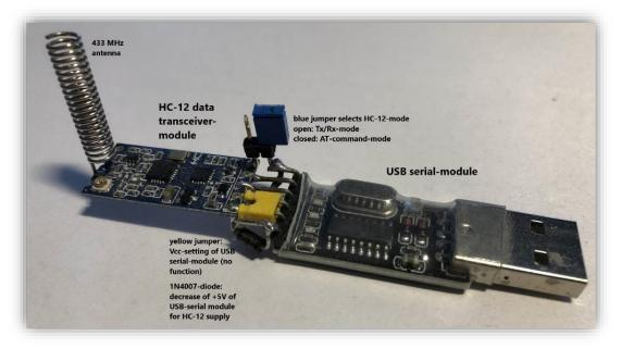
USB serial-module and HC-12 data transceiver-module (connections)
